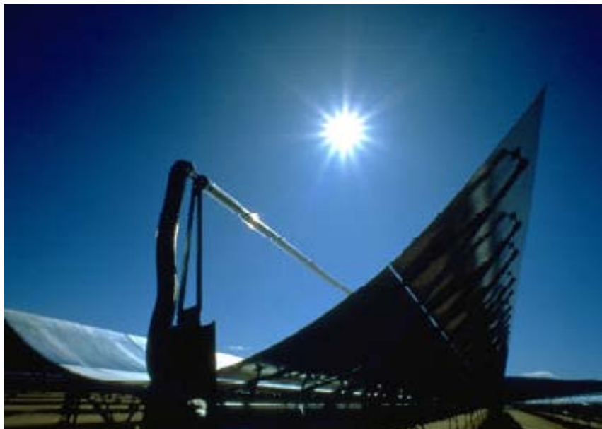
Figure 38 : Parabolic reflectors producing electricity used for hydrogen production
