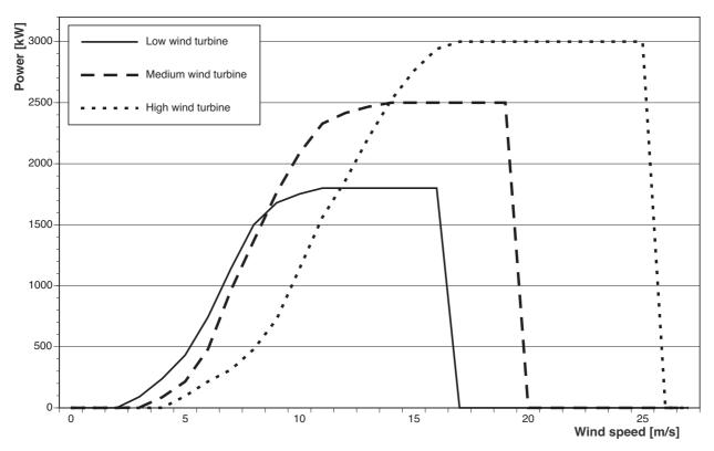
Source: ERJ. Figure 46 : Three wind turbine power curves
